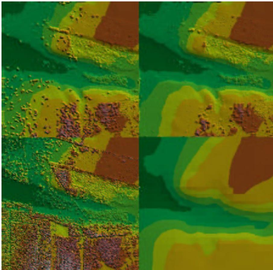
*Figure 5.1.3: Clockwise, starting at '6': unfiltered laserdata, first run, second run, old height model.*
