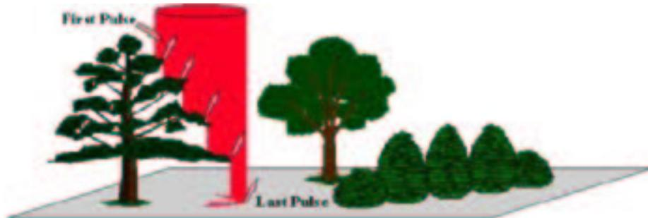
Figure 2.2.1: Reflecting behaviour of a laser pulse (source: [2]).
