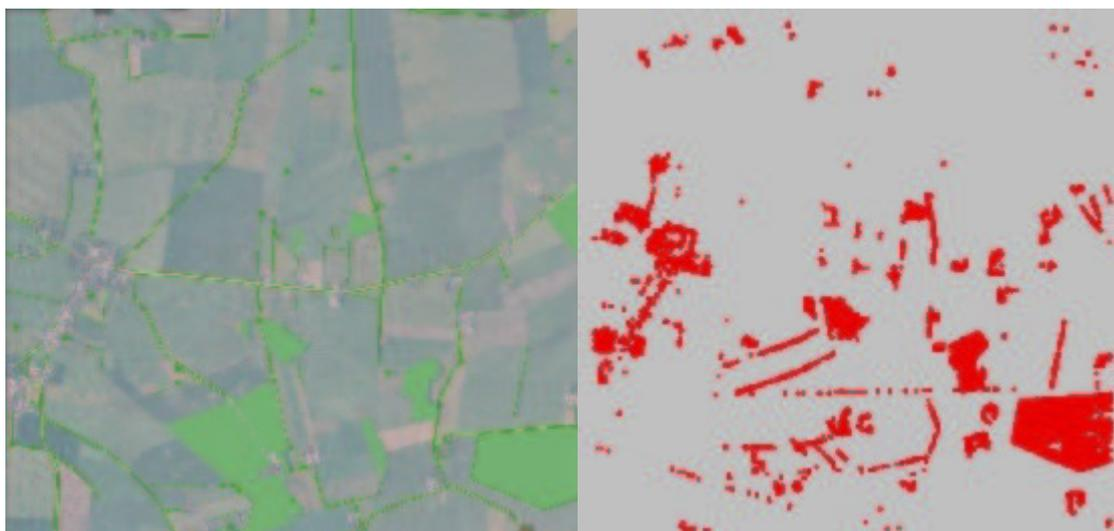
*Figure 5.3.3: Left, an aerial photograph with TOP10DK vegetation of the area on the right, where points are plotted in red with a height difference of at least 2 meters between the two pulse recordings.*
