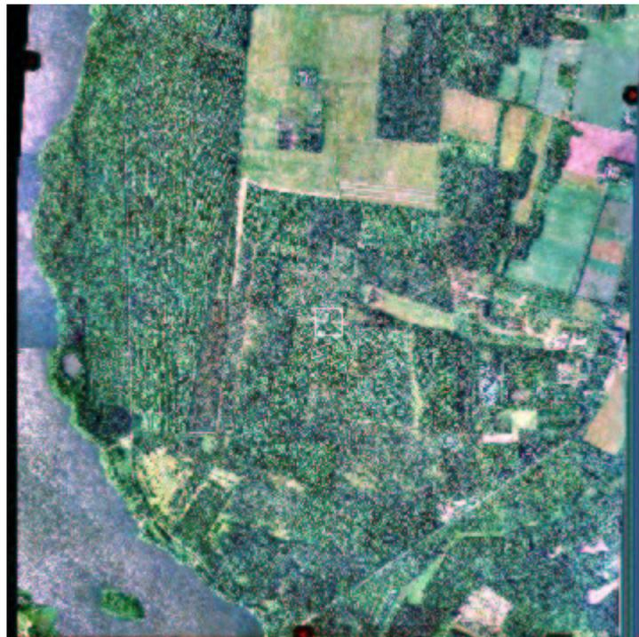
*Figure 3.4.3: Orthophoto with twists on both sides as result of the processing.*
