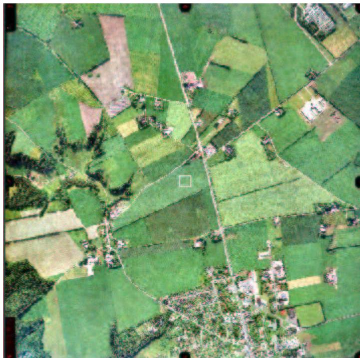
Figure 3.4.1: Scanned aerial photograph with the fiducial marks along the sides.
