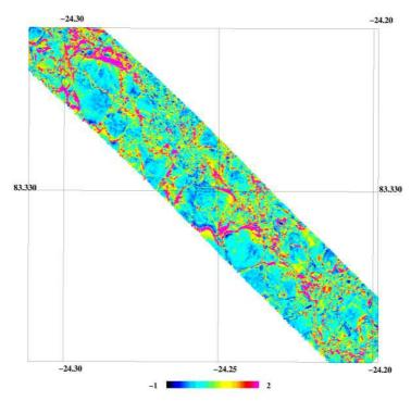
Fig. 16a. Example of section of sea ice with small floes and many pressure ridges (JD100). Heights are shown in meter above geoid, without fit to sea level. Width of scan approx. 300 m.
