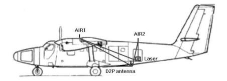
Fig. 13. GPS antenna offset vectors to laser and D2P radar
