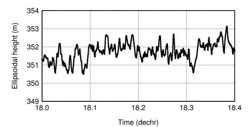
Fig. 9. Example of GPS aircraft height (JD 100), showing phugoid motion due to the autopilot feedback system. The regular phugoid motion is useful to check the timing calibration.
