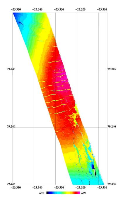
Fig. 17. Example of land ice heights by laser: Section of East Greenland ice sheet margin, showing crevasse field where lidar is seen to measure into crevasses. Ellipsoidal heights (meter).
