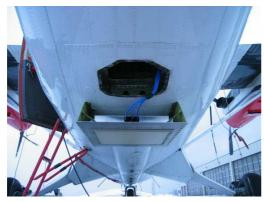
Fig. 5. D2P 13 GHz radar antenna
