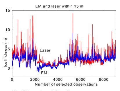
*Fig. 26.Comparison of EM and laser measurements. Length of profile approx. 30 km. April 11 flight.*
