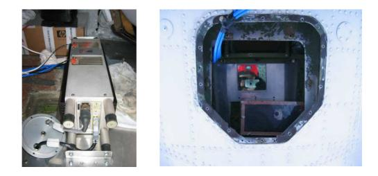
*Fig. 12. Riegl laser scanner with attached heating pads (left) and aircraft hole photographed from below, with scanner mirror, Canon Ixus camera in insulated box and connecting cables to D2P radar (right).*
