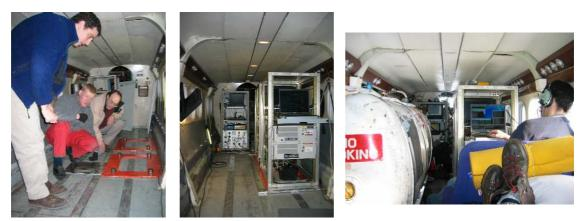
*Fig. 4. Installation of D2P radar racks (at right in pictures), KMS data logger (in back of pictures) and external ferry tank (at left in pictures) for extended 6 hr+ flight missions.*
