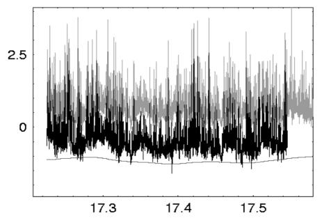
Fig. 18. Example of lowest level fitting of sea-ice lidar data. Black: lidar results; lower, smooth curve (grey): collocation minimum fit; grey (upper): freeboard heights. JD100.
