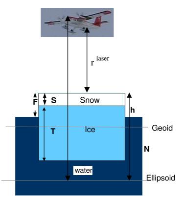
*Fig. 7. Principle of freeboard determination. The conversion of freeboard, F, to thickness, T, is approximately a constant (~6.0 - Wadhams, 2000) depending on densities and snow depth, S.*
