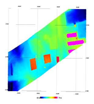
Fig. 14. Laser scan over Kangerlussuaq hangar, measured by GPS for calibration of offset angles.
