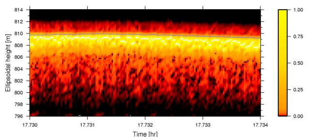
*Fig. 29. D2P signal power (color scale) and lidar (blue) over Austfonna icecap.*
