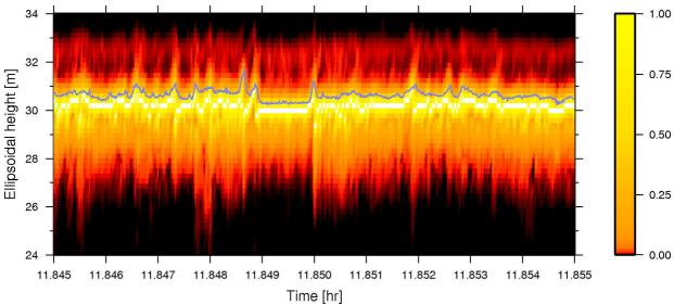
Fig. 30: D2P signal power (color scale) and lidar (blue) of sea-ice near Polarstern (April 15 flight)
