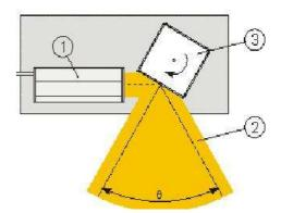
*Fig. 11. Scanning lidar principle. A laser (1) provides a swath (2) by reflection in a rotating mirror (3)*
