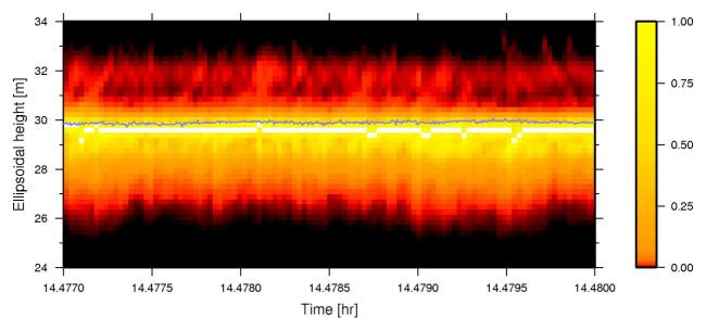
*Fig. 28: Comparison of D2P signal power (color scale) and lidar (blue) over open water and thin ice in Isfjorden just north of Longyearbyen, Svalbard.*
