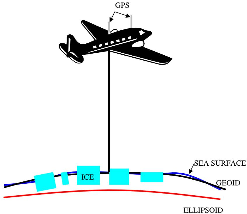
Figure 12. Airborne laser altimeter measurement principle.
