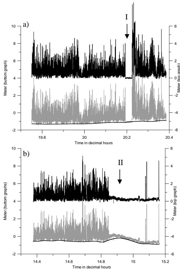
Figure 19. Example of height, freeboard and filter data. Grey curve: Freeboard heights from the equation above. Bottom black curve: Estimated sea surface used for filtering. Top black curve: Corrected freeboard heights after filtering (refers to right hand y-axis). Adapted from Hvidegaard and Forsberg (2002).
