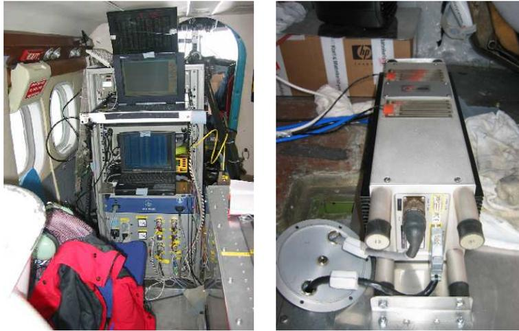
Figure 8. Photographs of the installation. Left: Rack with power conditioner, laptops, and GPS receivers. Right: Laser scanner
