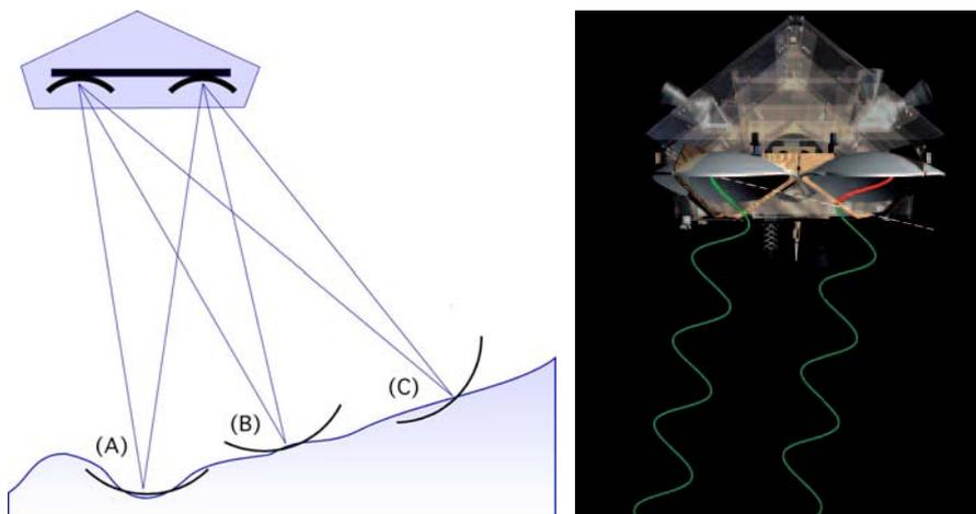
Figure 3. Illustration of SARin mode. Off nadir reflections will have different range between the surface and the two antennas shown as the red part of the signal on the figure seen to the right.
