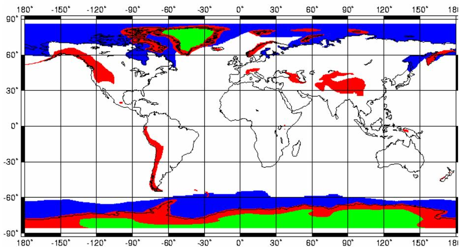
Figure 4. Example of the mask used for the different operation modes. Green: LRM, red: SARin mode and blue: SAR mode (ESA).
