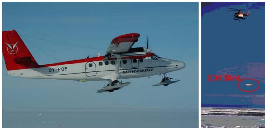
Figure 25. Photographs of the two aircrafts, the Air Greenland Twin-Otter and a helicopter carrying the HEM-bird as a sling load.
