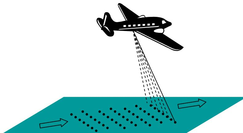
Figure 10. Laser scanner principle.
