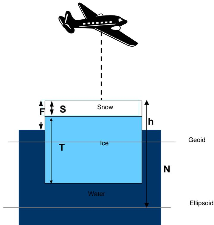
Figure 18. Principle of freeboard determination
