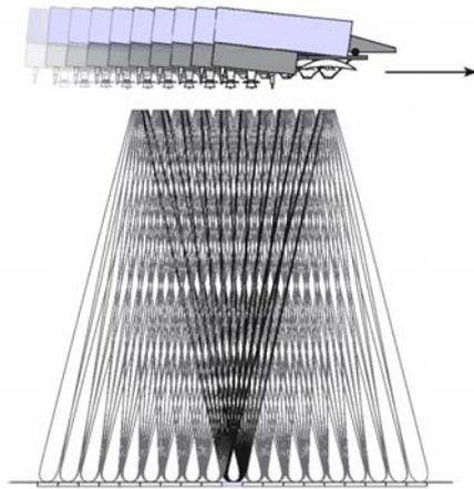
Figure 2. Illustration of the Doppler technique used for the synthetic aperture processing (ESA).
