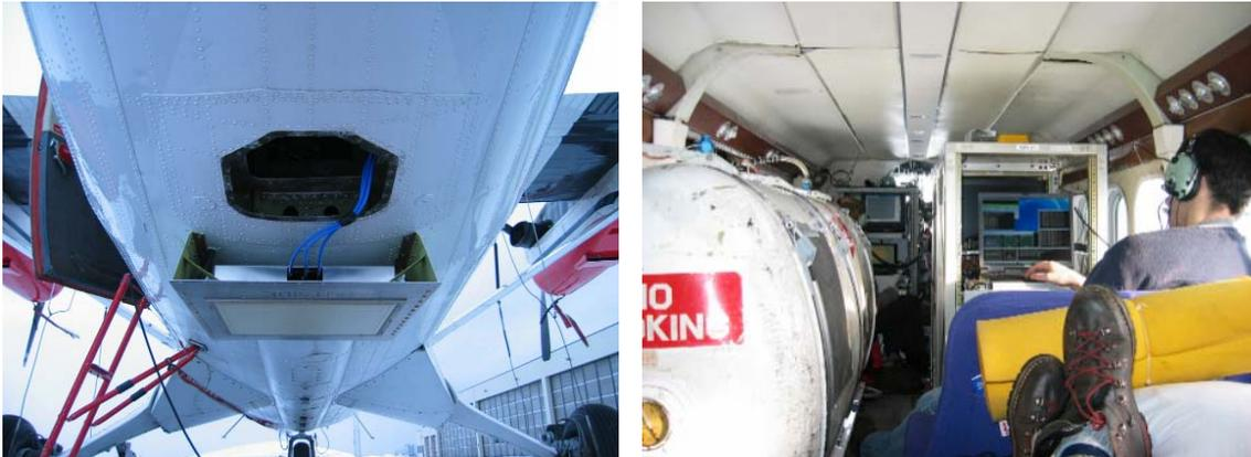
Figure 11. Photographs of D2P system. The antenna is seen to the left and the racks with the radar and data storages system from the cabin of the Twin-Otter is seen to the right.
