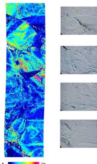
Figure 15. Examples of output sea ice elevation data from the laser scanner (2003 CRYOVEX survey). To the left is shown photographs from the nadir looking camera that was mounted next to the laser scanner.
