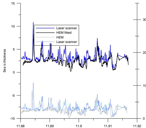
Figure 26. Small section of coincident HEM and scanner data: Example of data comparison showing high match of the features between the laser scanner derived sea ice thickness (blue) and the HEM determined thickness (black) after a small adjustment (top graphs) in addition to the drift corrected data (bottom graphs) (From Hvidegaard et al. 2005).
