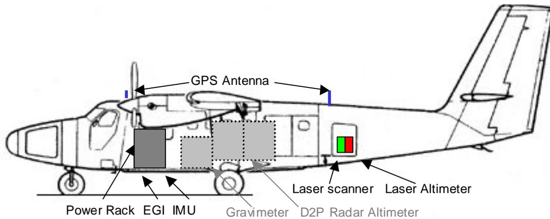
Figure 9. Sketch of how the instruments are mounted.
