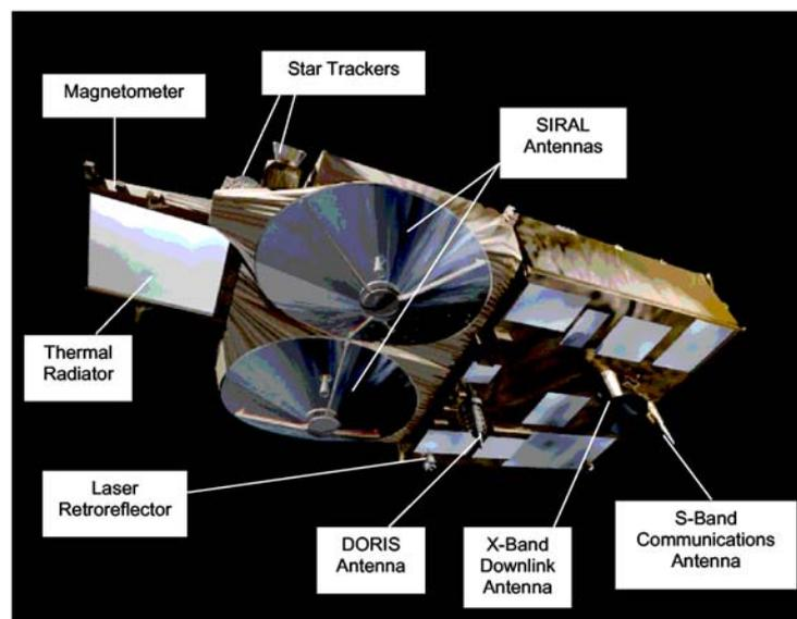
Figure 1. Illustration of CryoSat showing the instruments (Courtesy ESA).
