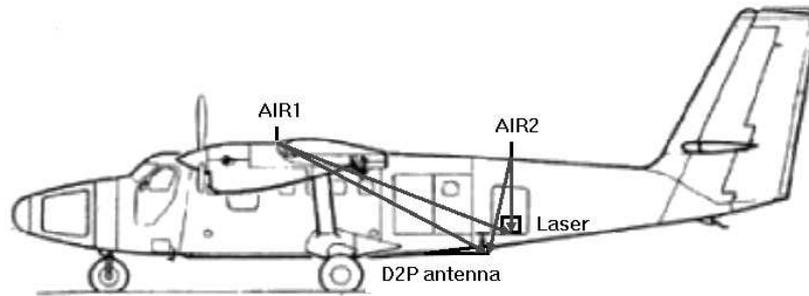
*Fig. 13. GPS antenna offset vectors to laser and D2P radar*
