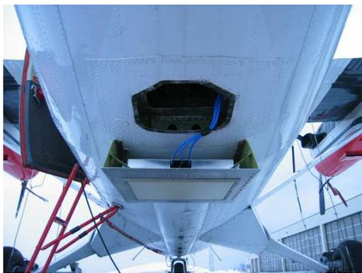
*Fig. 5. D2P 13 GHz radar antenna*
