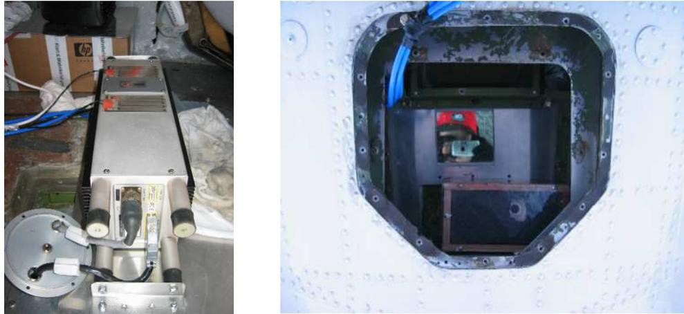
Fig. 12. Riegl laser scanner with attached heating pads (left) and aircraft hole photographed from below, with scanner mirror, Canon Ixus camera in insulated box and connecting cables to D2P radar (right).
