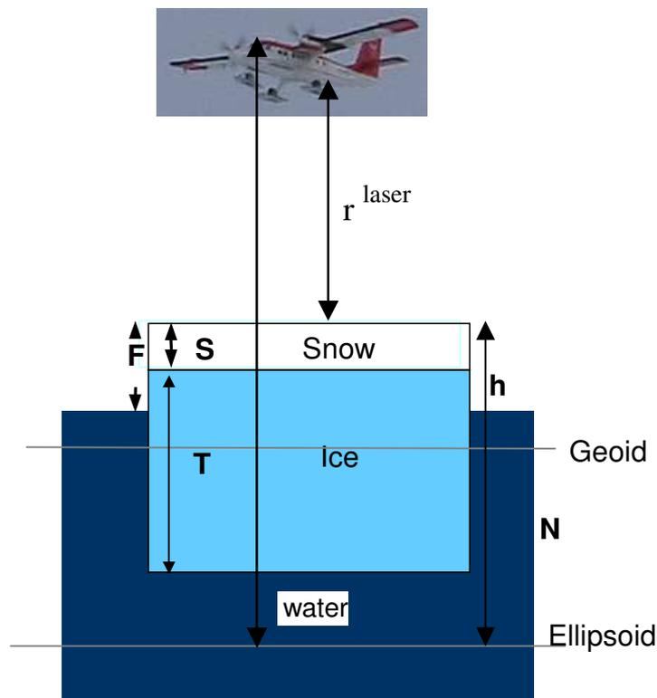
*Fig. 7. Principle of freeboard determination. The conversion of freeboard,  $F$ , to thickness,  $T$ , is approximately a constant ( $\sim 6.0$  - Wadhams, 2000) depending on densities and snow depth,  $S$ .*
