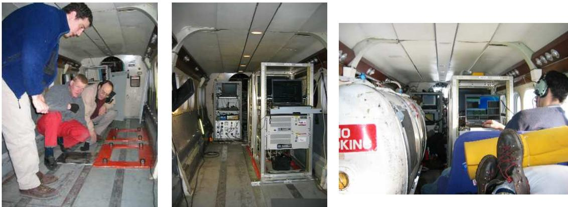
*Fig. 4. Installation of D2P radar racks (at right in pictures), KMS data logger (in back of pictures) and external ferry tank (at left in pictures) for extended 6 hr+ flight missions.*
