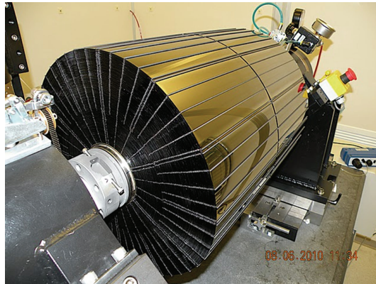
FIGURE 2: Picture of FM0 mounted on the assembly machine on the day of completion in August 2010. Picture courtesy of Todd Decker.
