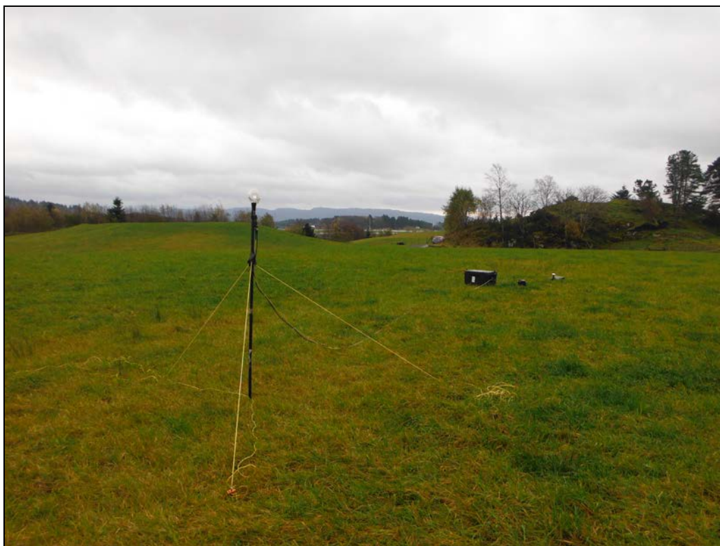
Figure 3: Magnetic Base Station A Installation
