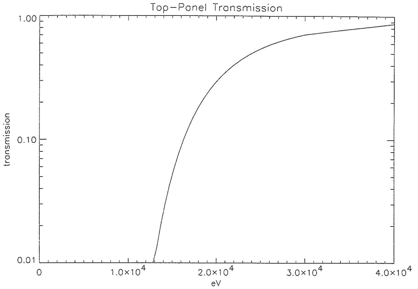
Figure 2: Transmission of X-rays through Top Panel
