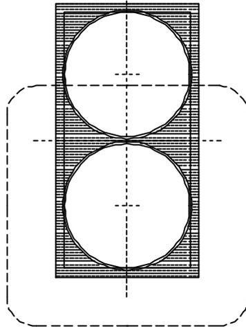
**Figur 1** JEM-X Mask Support Panel with indication of Collimator FOV.**3) Contributions from the peripheral areas.**
