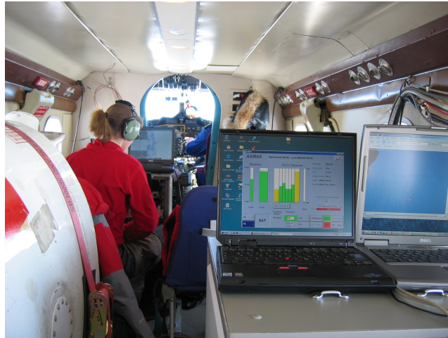
(a) The ASIRAS control PC inside the cabin during survey.
