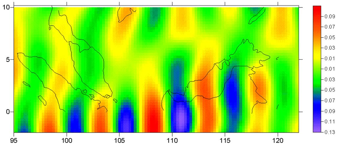
Fig. 8. Difference between GRACE models GGM01S and GGM02S to degree 80 in the Malaysian region. The N-S lineations are typical of GRACE data errors. The present errors will be inherited directly in East Malaysia (where degree 80 was effective cut-off for influence of local gravity data), but not in West Malaysia (where a cut-off of 40 was used in the kernels).
