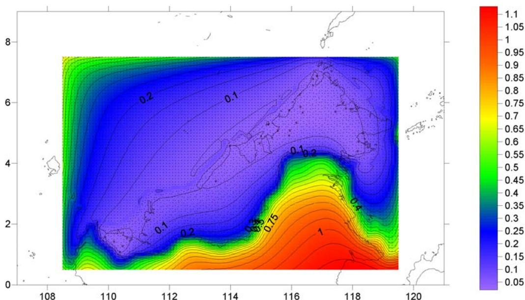
**Fig. 6a.** Collocation geoid error estimates in East Malaysia. Unit meter.
