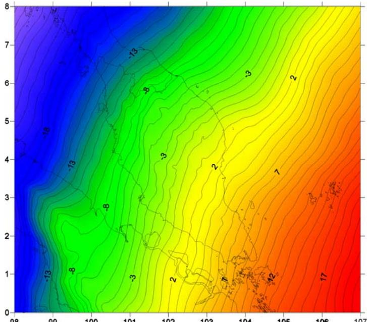
Fig. 4b. Final gravimetric geoid for peninsular Malaysia (WMG03C). Contour interval 1 m.
