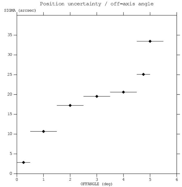
**Fig. 7.** The Crab position scatter ( $\sigma$ ), in units of arc-seconds, as a function of off-axis angle in degrees. This scatter in relative position determination represents the absolute positioning capability of JEM-X, once systematic are fully understood.
