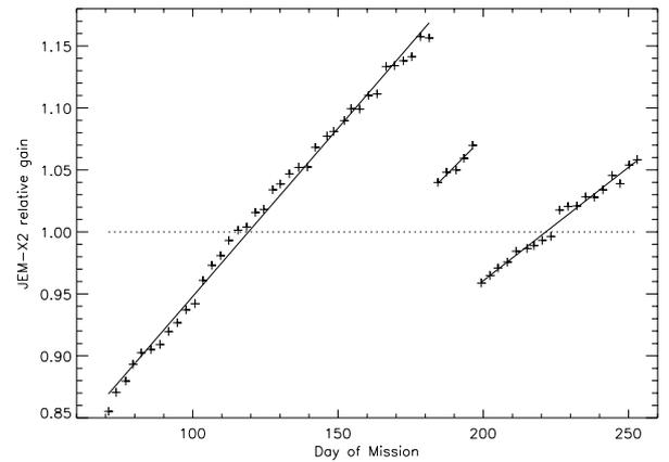
**Fig. 16.** The relative gain of JEM-X2 as a function of time (day of mission), normalized to the value during the Crab calibration in Feb. 2003. The plot covers the period until the end of June 2003. We initially observe a  $\approx 1\%$  increase per 4 days. The jumps indicate the lowering of the high voltage setting by 1 step (10 Volts), corresponding to a decrease of 12–13% in gain.
