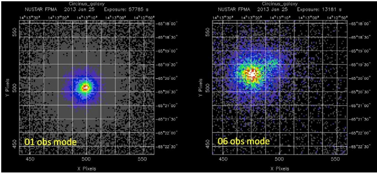
**Figure 5: NuSTAR FPMA sky images of the Circinus Galaxy (obsID 60002039002) for observation modes 01 (left) and 06 (right). In the mode 01 image, derived from CHU4 data, the target appears as a point-like source, while the mode 06 image shows multiple centroids from the same target due to the poor aspect reconstruction and the switching between different CHU1/CHU2/CHU3 combinations.**
