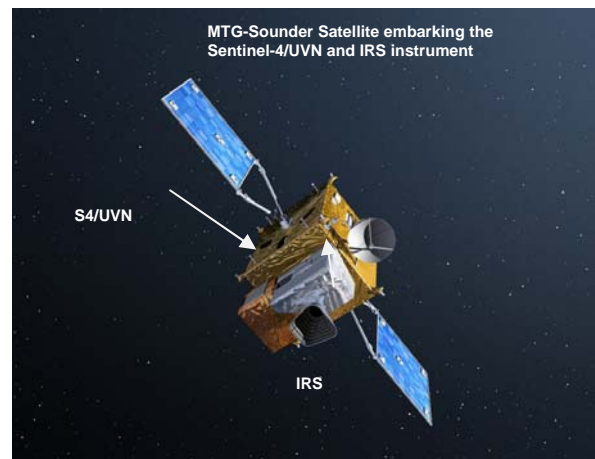
Figure 2. MTG-S with the Sentinel-4/UVN and Infra-Red Sounder (IRS)
