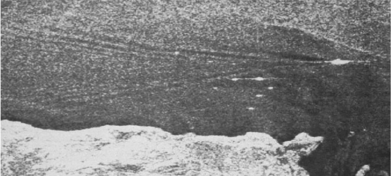
Figure 5. Radar image of the Sir Tristram wake. Ship speed is 2.0 m/s (from [8]). The bright spots to the right of the centre are the locations of sensor buoys.
