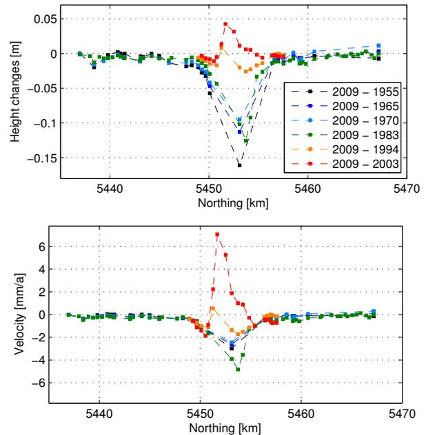
Figure 4. Height changes (top) and velocities (bottom) along a levelling line in the Northern part of the URG w.r.t. the last measurement epoch. The height of the starting point is kept fix.
