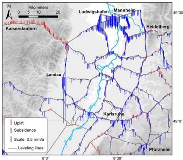
Figure 3. Vertical displacement rates in the Northern URG from kinematic adjustment of levelling data.
