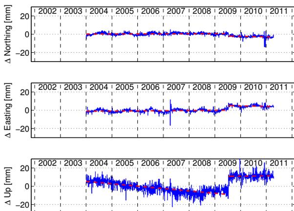
Figure 8. Time series of the local topocentric coordinate components (blue) for GURN site Landau. In addition, estimated regression lines (red) are shown.
