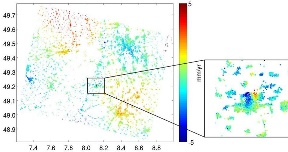
Figure 6. LOS displacement rates in the Northern URG without slave atmosphere estimation. The inset covers the city of Landau with the oil extraction field.
