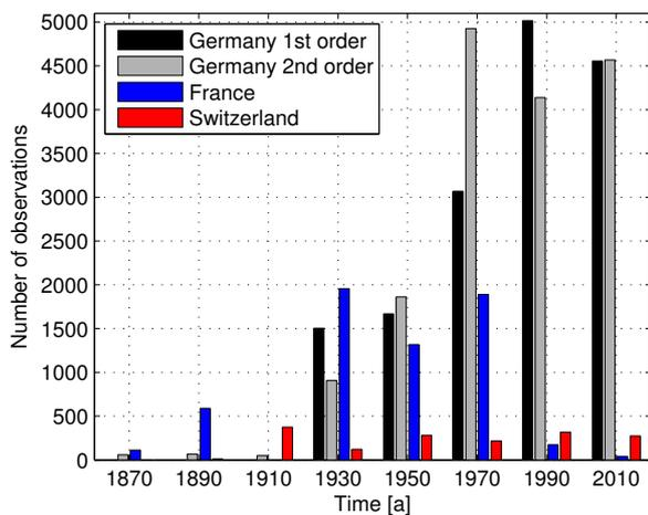
Figure 2. Temporal distribution of levelling observations at repeatedly measured benchmarks for different groups of data.
