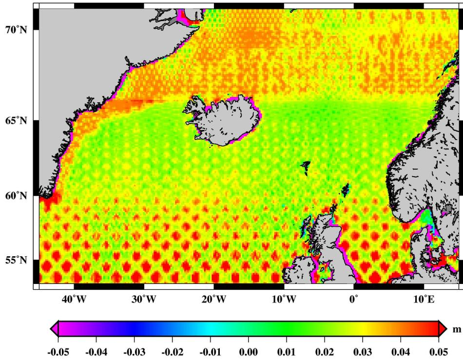
Figure 8. Difference between error files for KMS03 and CLS01 MSS (KMS minus CLS).
