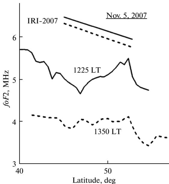
**Fig. 3.** Latitudinal dependence of the critical  $foF2$  frequency measured on November 5, 2007, over Sakhalin Island.
