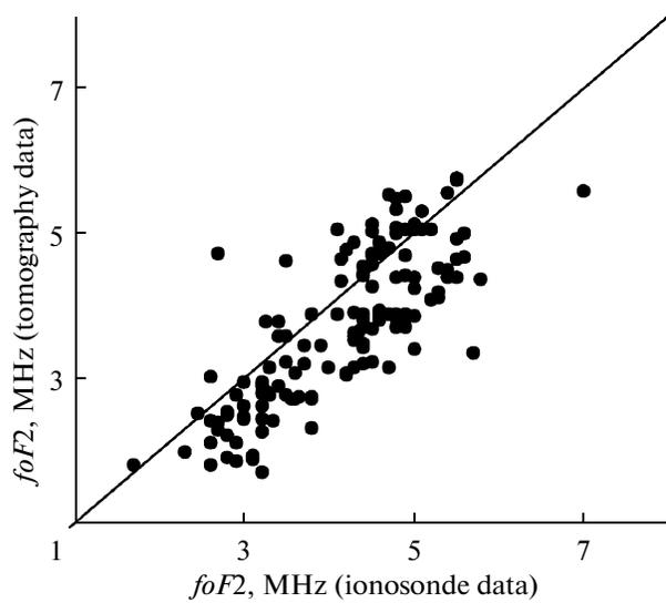
Fig. 2. Comparison of the critical frequency *foF2* values obtained as a result of ionospheric tomography with the data of a Wakkanai ionosonde.
