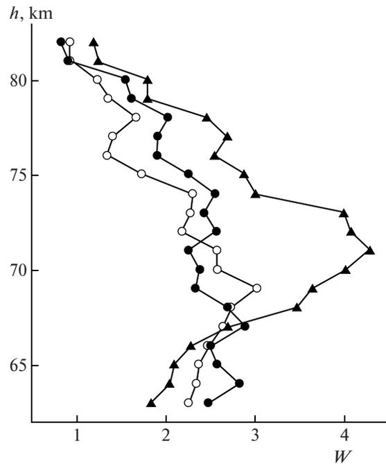
Fig. 5. Ratio of the  $[e](h)$  profiles (from Fig. 2) to the  $[e](h)$  profile obtained during the TC active phase (flight 50).
