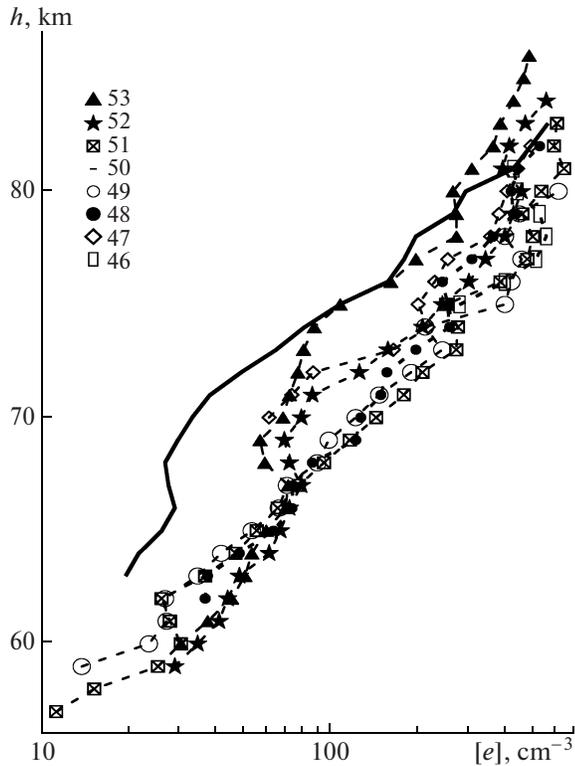
Fig. 1. Vertical profiles of the electron concentration  $[e](h)$  obtained in May–June 1985 at the Thumba rocket site.
