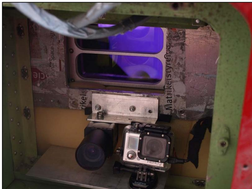
Figure 14 Camera installation of nadir-looking cameras for CryoVEx 2016; uEye (left) and GoPro (right).
