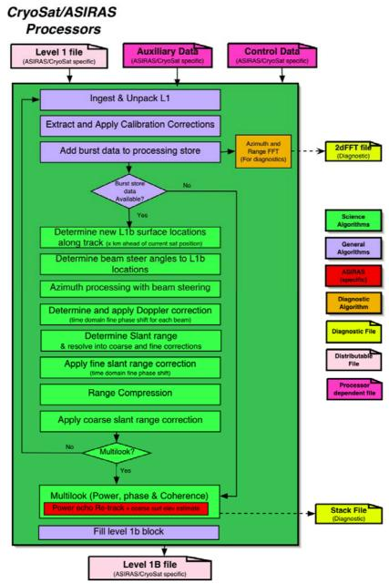
Figure 10. ASIRAS processing scheme.
