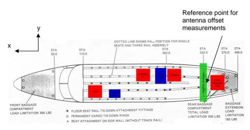
Figure 2. Sketch of instrument installation in the Air Greenland Twin Otter.
