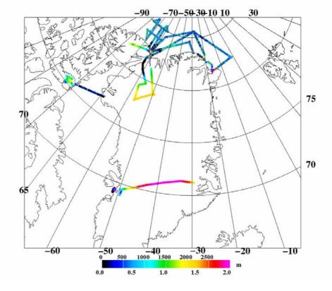
*Figure 9. Overview of delivered laser scanner data, colour coded separately for sea ice and ice caps. Note that the sea ice data has been filtered to heights relative to local sea level.*
