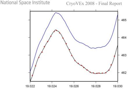
Figure 4. Draping of high rate INS derived heights (blue) onto precise GPS heights (red) to get high rate precise heights (black).
