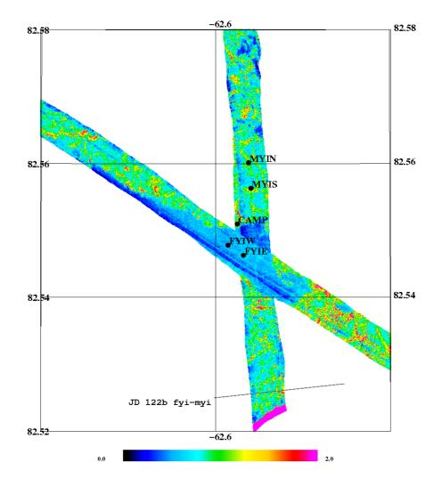
Figure 14. Stacked laser scanner swaths from sea ice validation sites near Alert (heights are freeboards relative to the local sea level). Over-flight performed on May 1.
