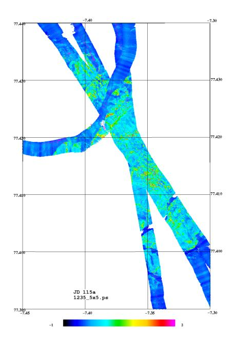
*Figure 18. Laser scanner data from the KV Svalbard over-flight. Note that the sea ice has moved significantly during the survey (the crossing track has been observed last).*
