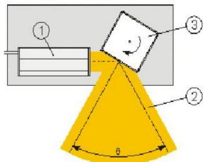
Figure 5. Sketch of laser scanner principle (1) Laser and photodiode assembly (2) Swath pattern (3) Rotating mirror.
