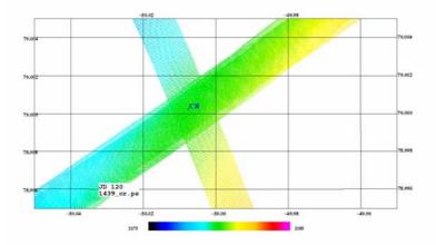
*Figure 13. Stacked laser scanner swaths of the over-flights of the ICE2 validation site April 29.*
