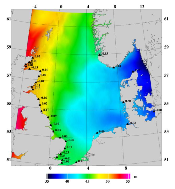
Fig. 4. The DTU10 MSS, with differences to mean sea level  $H_{ELL}$  at available tide gauges. An offset of 90 cm has been applied to make the BLAST MSS surface. It is obvious that the local heights of mean sea level in the ETRF datum are very noisy, affected by local effects and errors, so it does not make sense to propagate these offsets into the North Sea.
