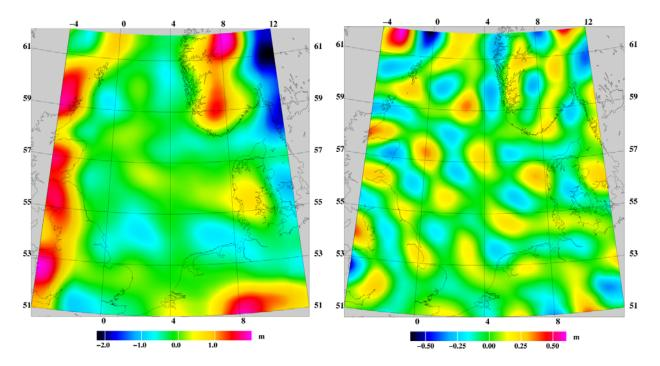
Fig. 8. Left: Filtered EGG geoid (harmonic band 60-150), and difference to the "timewise" GOCE geoid in the same band. Note the difference in colour scale.
