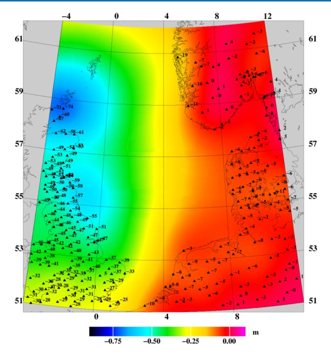
Fig. 3. The modelled difference surface between EVRF2007 and the EGG08 geoid. The surface "EVRF-DIF" has been modelled using least-squares collocation with a correlation length of 300 km and a standard deviation of 5 cm, to ensure a smooth surface [Updated Aug 2011 to diminish some geogrid artefacts in the central North Sea].
