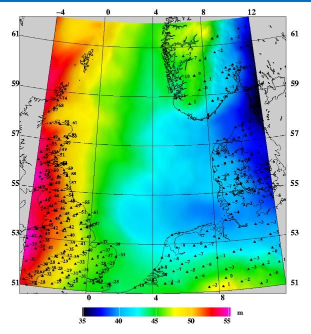
Fig. 2. Height differences between GPS-levelling geoid ( $H_{ELL}$ - $H_{EVRF}$ -N) in cm, overlain on the EGG2008 geoid. Because of the apparent tilt of the UK levelling, it has been decided to use the EGG2008 VD as the fundamental BLAST VD, both on land and at sea.
