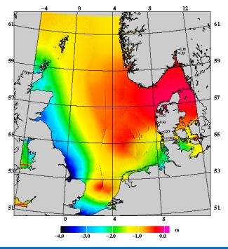
Fig. 8. The BLAST LAT surface, based on the DTU10-FES04 updated model, and local LAT corrections offshore two regions in the UK (same as for the MDT) and the inner German Bight.
