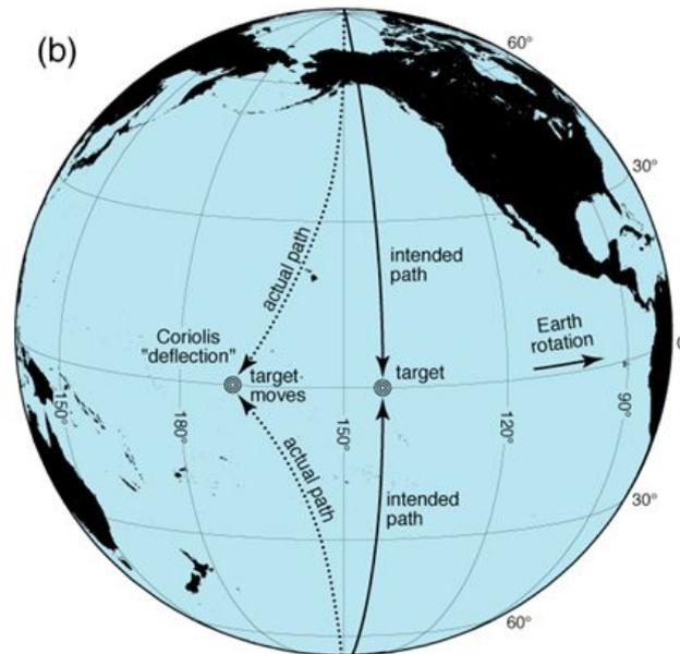
$f = 2 \Omega \sin \varphi$  is the "Coriolis parameter"
