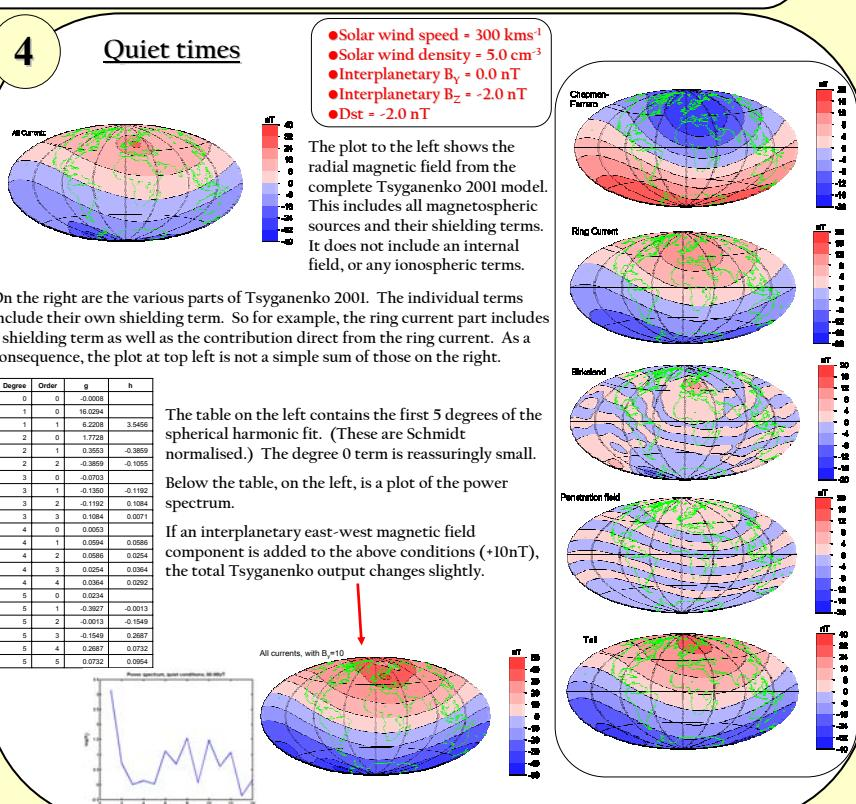
On the right are the various parts of Tsyganenko 2001. The individual terms include their own shielding term. So for example, the ring current part includes a shielding term as well as the contribution direct from the ring current. As a consequence, the plot at top left is not a simple sum of those on the right.
